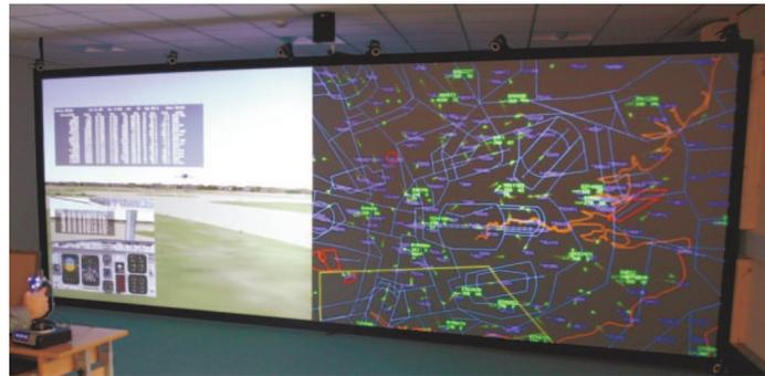
Figure 7. VEC 6m x 2.1m visualization screen showing outside world and air traffic situation
