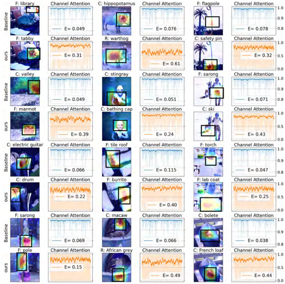
Fig. 7: Comparative Results between the SE-ResNet50 (baseline) and APA*-ResNet50 (ours) with respect to the activations (left) and the attention entropy (right). F,C,R denote frequent, common and rare samples from ImageNet-LT. Our method produces attention signals that have significantly larger entropy than the baseline for both frequent and rare classes.
