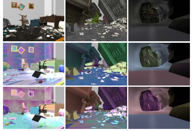
Fig. 5. Different robot’s views in our simulation of complex environments: collapsed city, natural cave, and collapsed house. Top row: RGB images from robot viewpoint in normal setting. Other rows: The same viewpoint when applying domain randomisation to the simulated environments.
