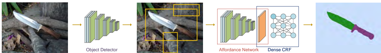
Fig. 2. An overview of our affordance detection method. From left to right: A deep network is first used as an object detector to generate the object bounding boxes that narrow down the region of interest. A second network is then used to produce feature maps from these bounding boxes. Finally, these maps are post-processed with dense CRF to improve the prediction along the class boundaries.
