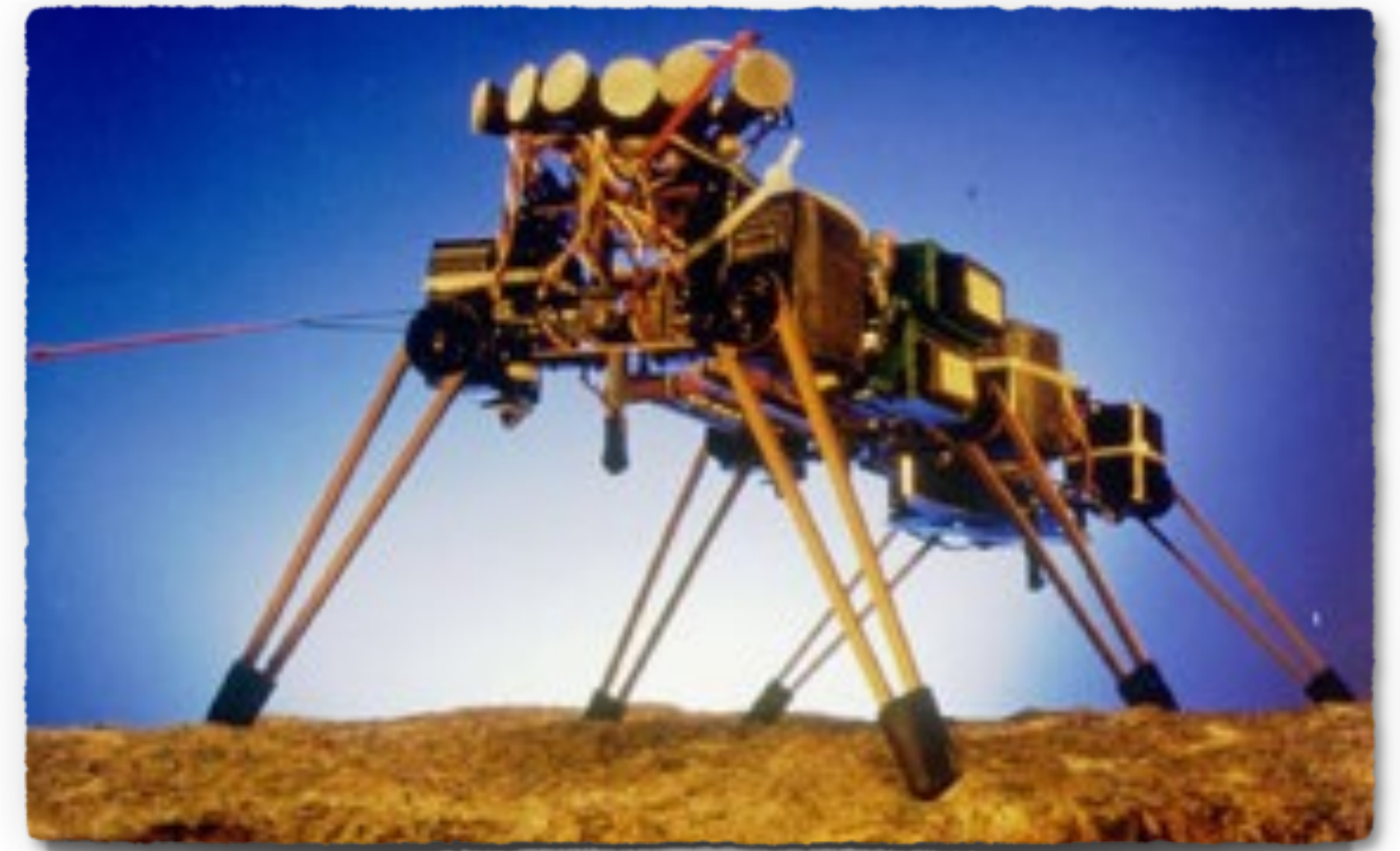
Rodney Brooks “subsumption architecture” was originally developed open Genghis
