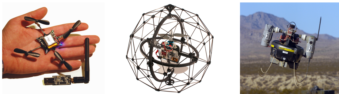
FIGURE 1.2: Various MAV platforms: The Crazyflie Nano [22], a 20 gram MAV platform (left); the Flyability Gimball [27], a coaxial rotor driven platform surrounded by a gimbal mounted protective cage for enhanced collision protection (middle); and the Honeywell RQ-16 T-Hawk [81], a ducted fan Vertical Take-off and Landing (VTOL) MAV developed by the United States military (right).
