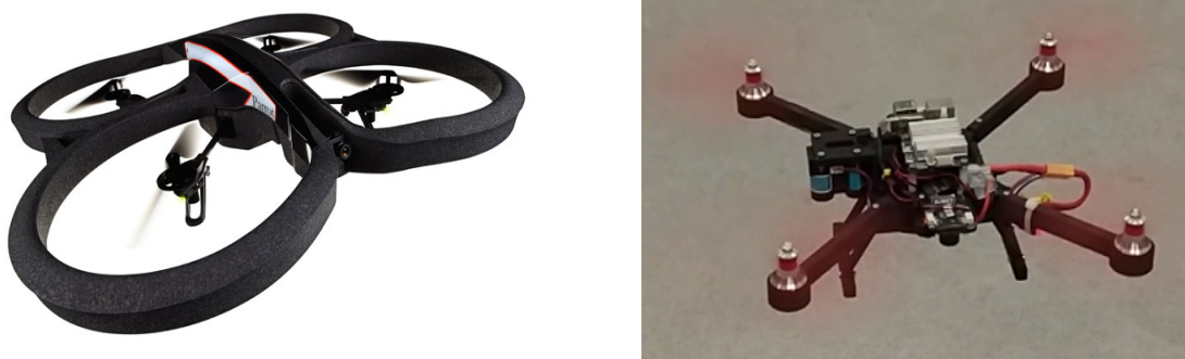
FIGURE 1.4: The MAV platforms used for the work presented in this thesis, the standard Parrot AR Drone (left) and a custom 3D printed, MAV platform (right).
