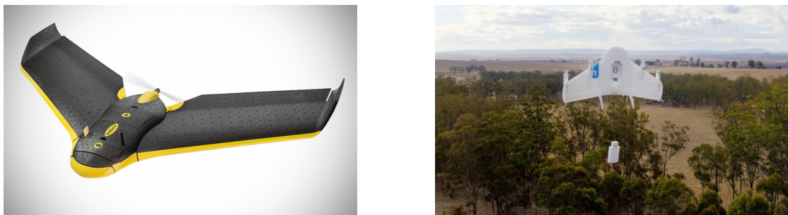
FIGURE 1.1: Small UAS: The SenseFly eBee (left) and Project Wing by Google (right) a VTOL craft delivering a package in the Australian outback. Image credits to Sensefly and Google respectively.
