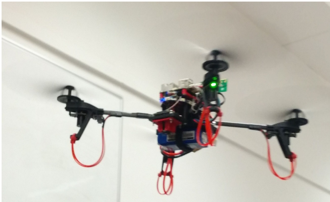
FIGURE 6.7: The first DCTAM hardware platform based on the AR.Drone frame and PX4 flight controller.
